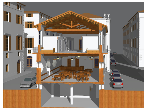
Figure 4. Cut-away section: top floor housing, ground floor (raised) dining, lower level kitchen/service. Author
